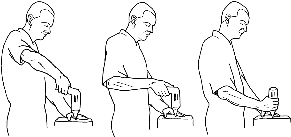
Figure 8. Pistol handle with an angle between the handle and the rest of the tool of 110^\circ and 90^\circ and a straight tool used when processing of a horizontal surface of a work-piece lying on a workbench. The straight tool provides the best working position and 110^\circ gives the worst.
