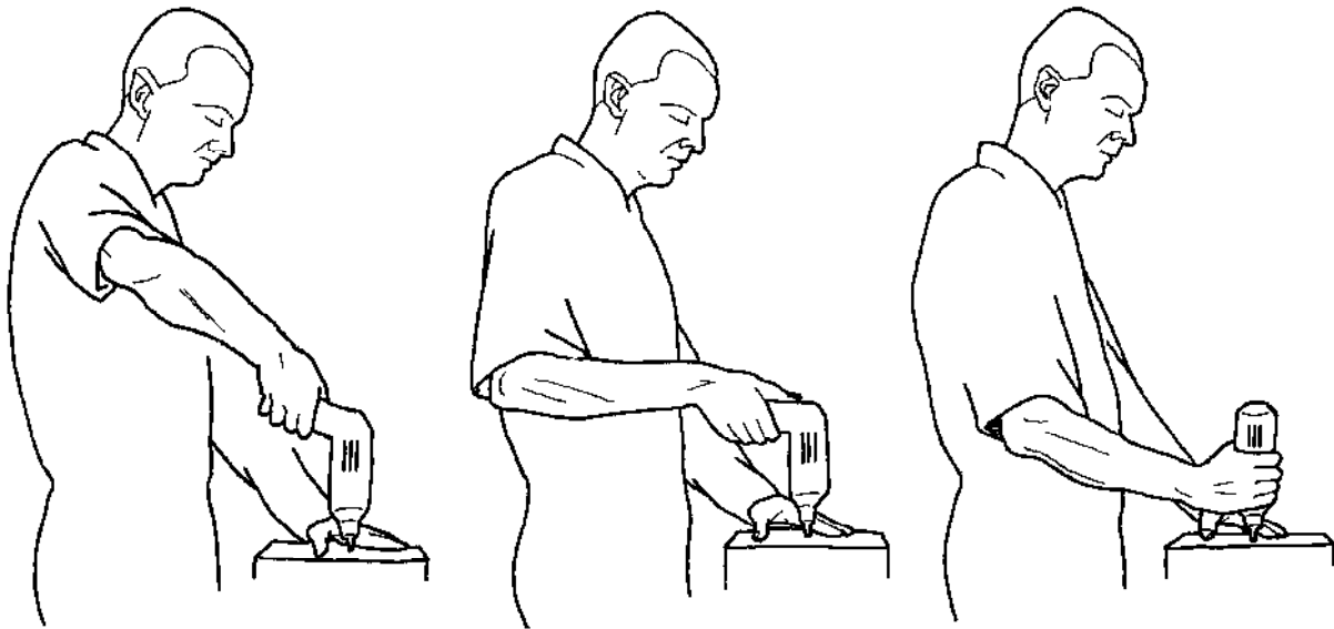
Figure 8. Pistol handle with an angle between the handle and the rest of the tool of 110° and 90° and a straight tool used when processing of a horizontal surface of a work-piece lying on a workbench. The straight tool provides the best working position and 110° gives the worst.
