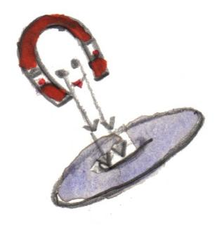
The hard drive and the disk drive stores all bits on magnetic disks. The magnetic disks are full of posts where the processor can put bits. Each station has eight slots. Each slot can be either magnetic or not magnetic. The processor can change from one to the other by means of electric magnets.
