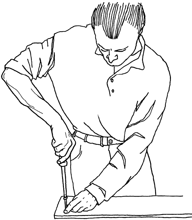
Figure 9. A screwdriver which is not suitable for the task, since it forces the user to lift the upper arm outwards.
