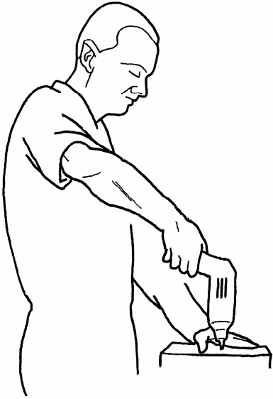
Figure 8. Pistol handle with an angle between the handle and the rest of the tool of 110^\circ and 90^\circ and a straight tool used when processing of a horizontal surface of a work-piece lying on a workbench. The straight tool provides the best working position and 110^\circ gives the worst.
